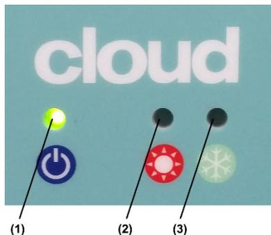
The first LED (1) indicates that the MATOS Monitoring system is powered.
