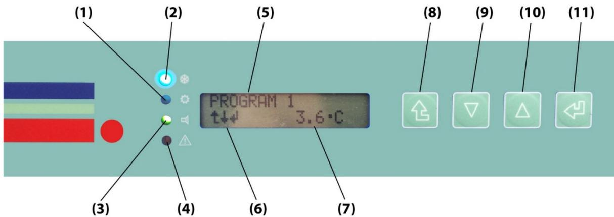
1. Heating system signal (Orange LED)
